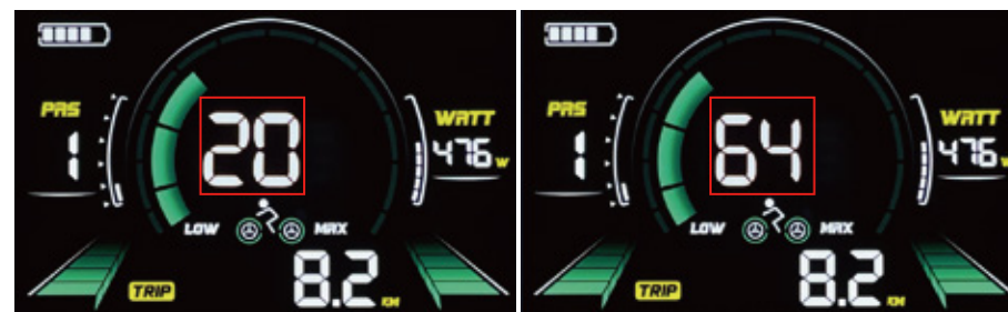
Figure 5-9: Speed limit Display Interface
