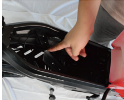
2. Slowly lower the groove on the battery along the fixing bracket
