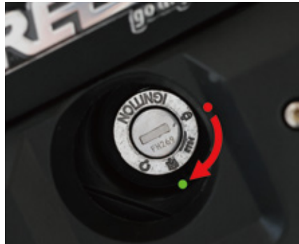
4. Insert the key and rotate clockwise to lock the battery.
