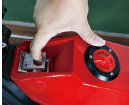
1. Lift the pull ring to open the battery cover
