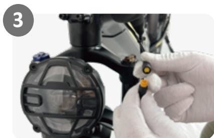
3. Connect the headlight cable and make sure the two arrows on the connector aligned.
