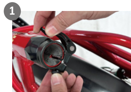
1. Open the quick release lever by swinging the lever open and outward fully.
