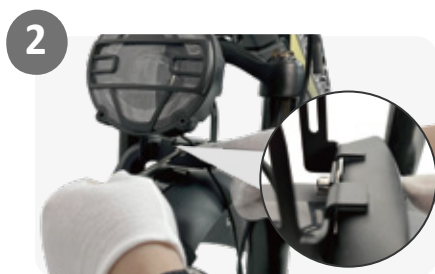
2. Pass the bolt through the headlight mount hole to tighten fender and headlight.
